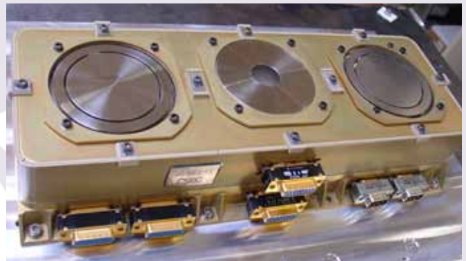
Flight model of the TPMU for Proba-2 satellite, planar sensors are placed on the top of the device
