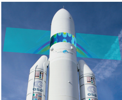
Visualization of the deformation of a thermal insulation panel and outer flux field on Ariane 5. Source: ESA & L.K. Engineering
